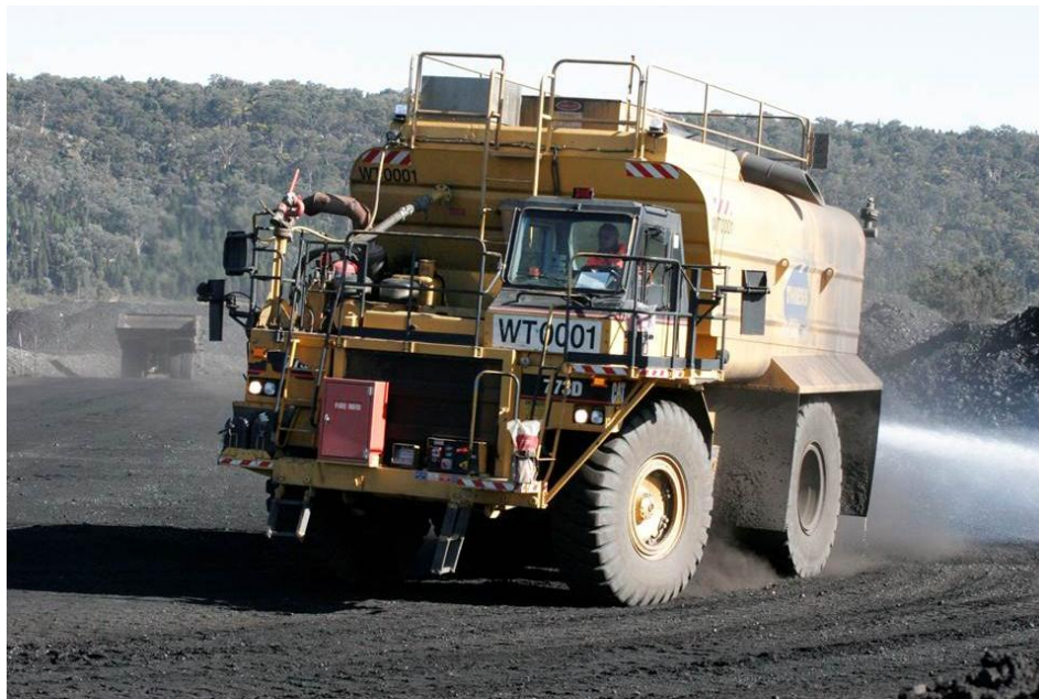
Figure 3: Watering of haul roads
