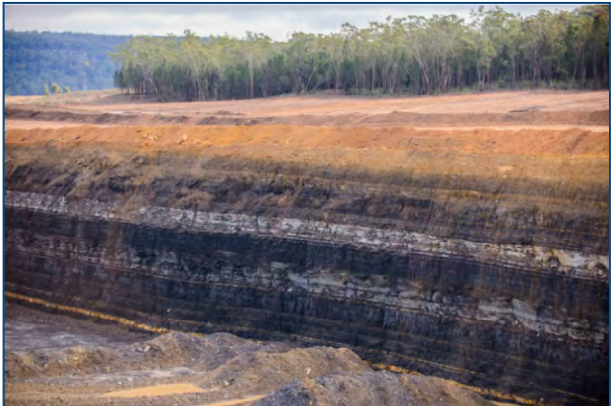
Plate 2: Pit Wall Showing Various Coal Plies and Shallow Overburden
