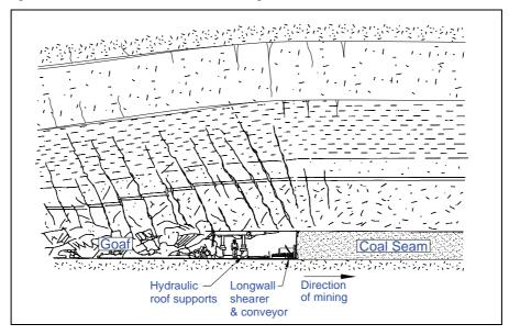
Fig. B. 1 Cross-section along the Length of a Typical Longwall at the Coal Face
