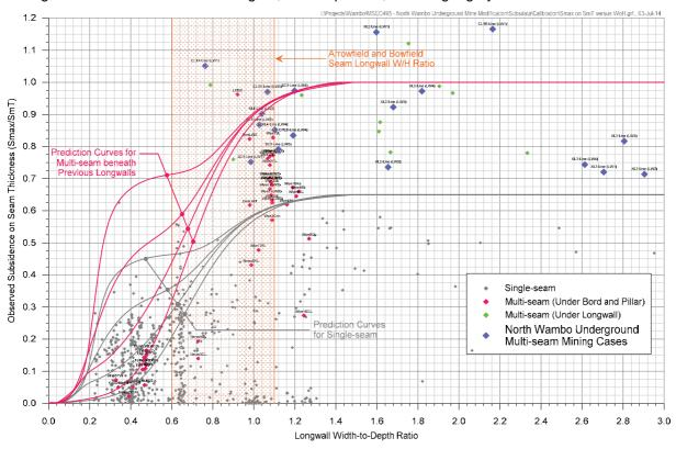
Fig. 3.1 Maximum Observed Subsidence versus Longwall Width-to-Depth Ratio for Historical Multi-seam Mining Cases
