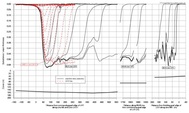
Fig. B. 2 Observed Subsidence Profiles at South Bulga Colliery
