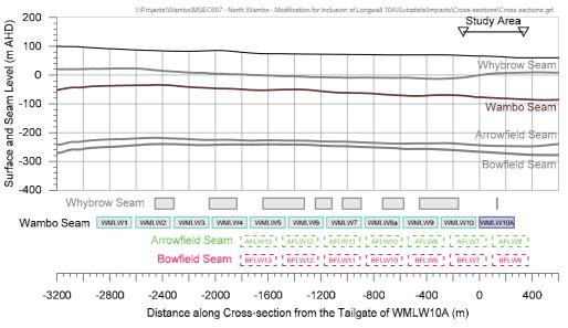
Fig. 1.2 Surface and Seam Levels along Cross-section 1
