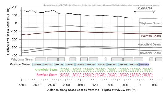
Fig. 1.3 Surface and Seam Levels along Cross-section 2
