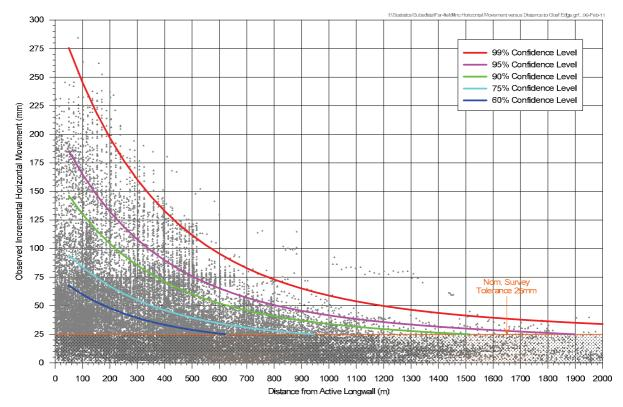
Fig. 4.3 Observed Incremental Far-Field Horizontal Movements
