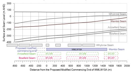
Fig. 1.1 Surface and Seam Levels along Long-section A
