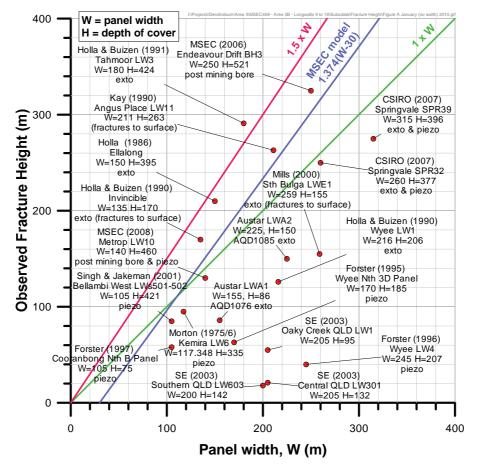
Fig. 4.9 Observed Fracture Heights versus Panel Width
