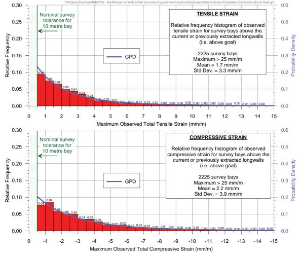
Fig. 2.1 Distributions of the Measured Maximum Tensile and Compressive Strains for Survey Bays Located Directly Above Goaf at the NWUM and Blakefield South Mine
