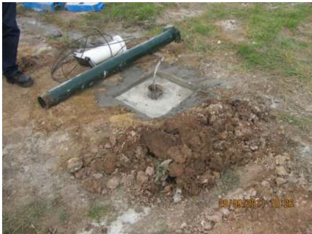
Plate 26 – view of a United drill hole that has been converted into a vibrating wire piezometer. .
