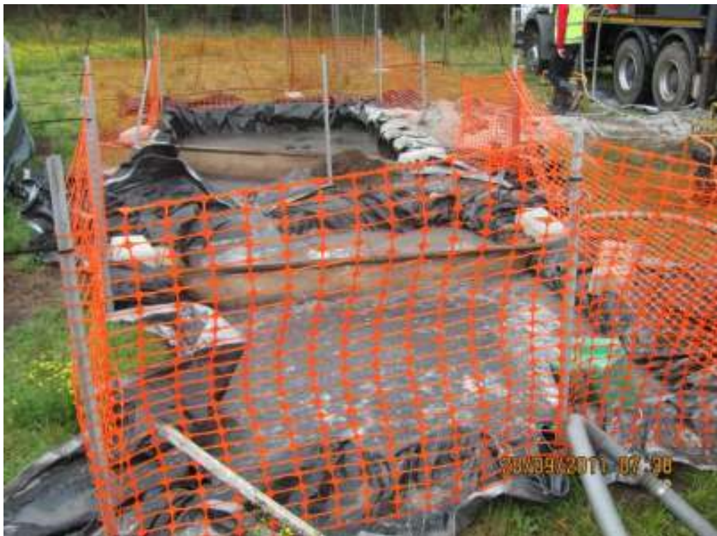
Plate 12 – view back to the active Wambo Drill Site (not within A444). GSSE observed that the sumps were nearly full and had insufficient freeboard in the event that a storm occurred.
