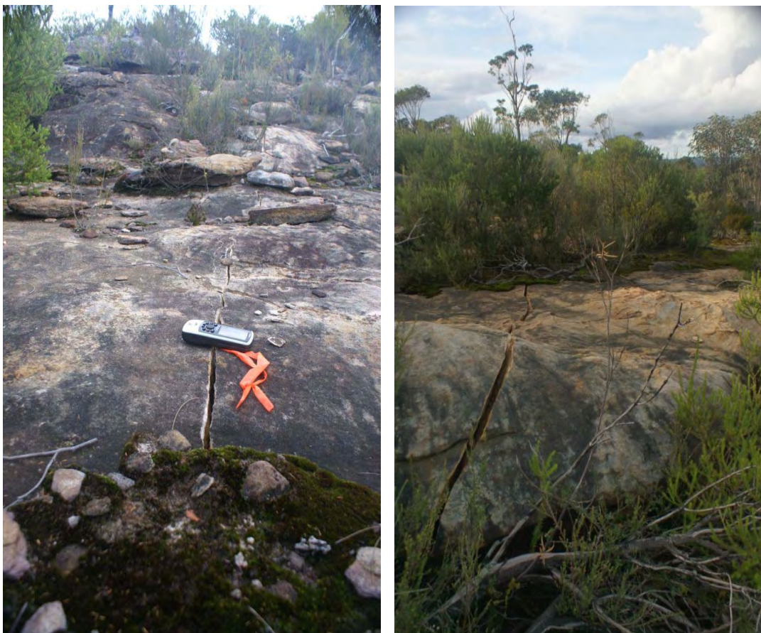
Plates 1 and 2: Surface Tension Crack above Longwall 18
