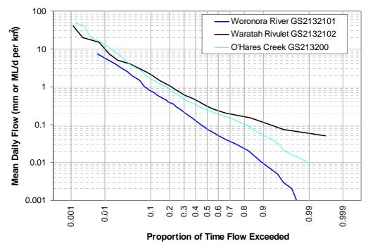
Figure 9 Flow Duration Curves – Waratah Rivulet, Woronora River and O'Hares Creek at Wedderburn
