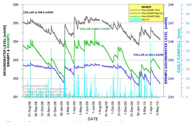
Figure 18 Perched Groundwater Hydrographs in Upland Swamps
