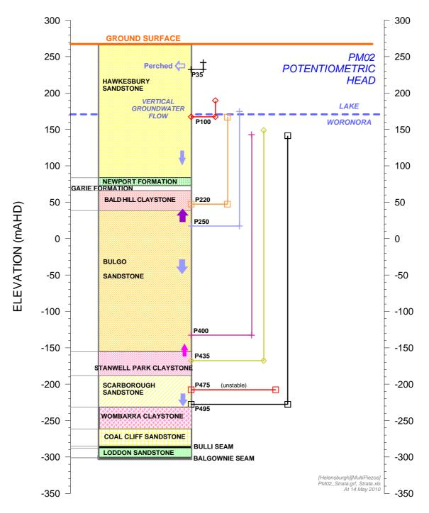
Figure 25 Vertical Groundwater Flow Directions, Relative Piezometer Elevations and Potentiometric Heads at Bore PM02 [at 14 May 2010]
