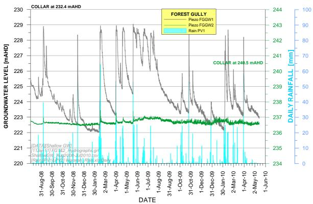
Figure 22a Shallow Groundwater Hydrographs along Forest Gully at FGGW1 and FGGW2
