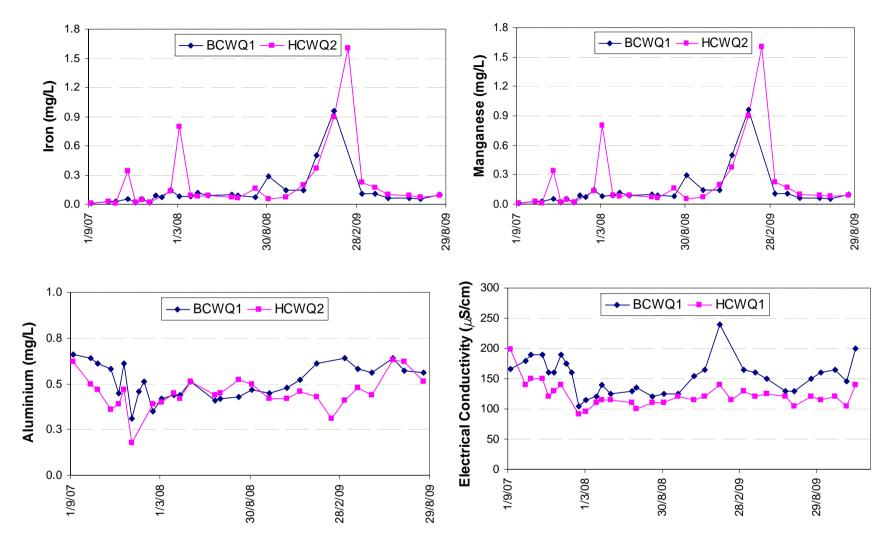
Figure 14 Water Quality Time Series – Bee Creek and Honeysuckle Creek Monitoring Sites
