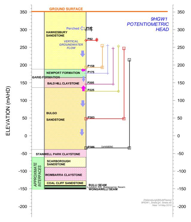
Figure 24 Vertical Groundwater Flow Directions, Relative Piezometer Elevations and Potentiometric Heads at Bore 9HGW1B [at 14 May 2010]
