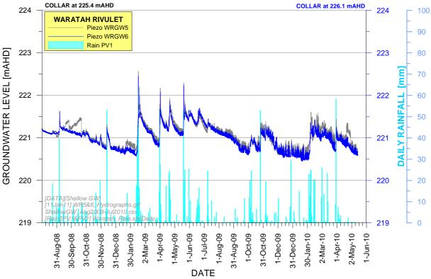
Figure 20c Shallow Groundwater Hydrographs along Waratah Rivulet at WRGW5 and WRGW6
