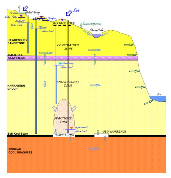
Figure 32 Conceptual Groundwater Model
