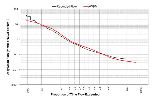
Figure 35 Recorded and Modelled Flow Duration Curves - GS2132102 Waratah Rivulet
