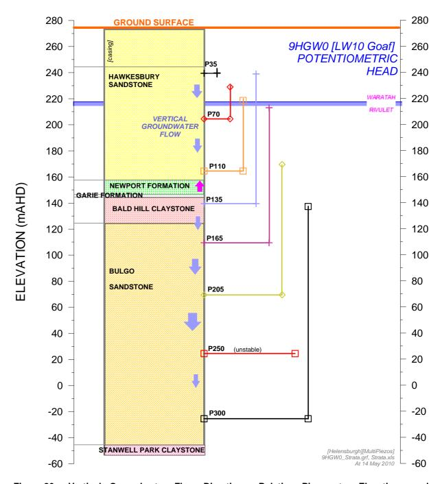
Figure 26 Vertical Groundwater Flow Directions, Relative Piezometer Elevations and Potentiometric Heads at Bore 9HGW0 (Longwall 10 Goaf Hole) [at 14 May 2010]
