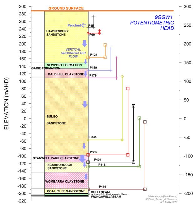
Figure 23 Vertical Groundwater Flow Directions, Relative Piezometer Elevations and Potentiometric Heads at Bore 9GGW1B [at 14 May 2010]
