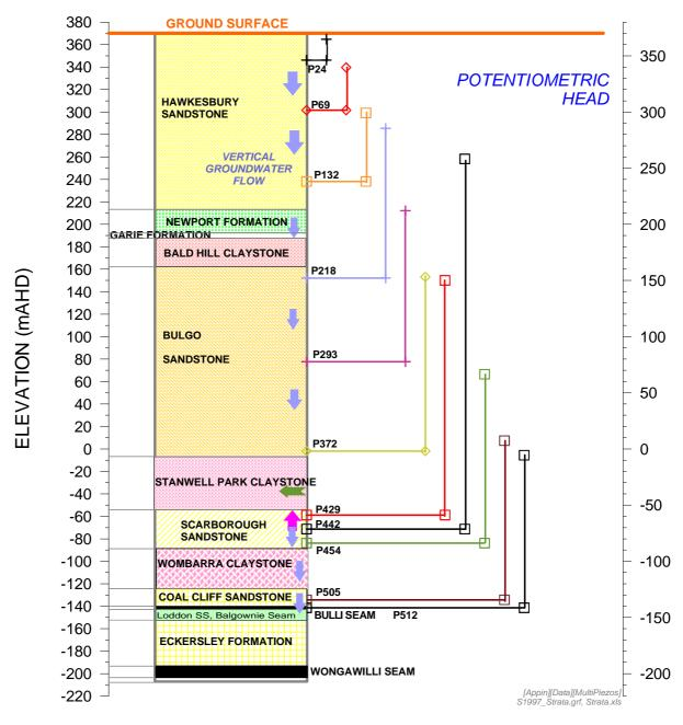
Figure 27 Vertical Groundwater Flow Directions, Relative Piezometer Elevations and Initial Potentiometric Heads at Bore S1997 at North Cliff [Sampled 15 June 2009]
