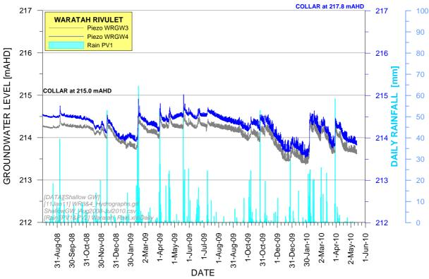
Figure 20b Shallow Groundwater Hydrographs along Waratah Rivulet at WRGW3 and WRGW4
