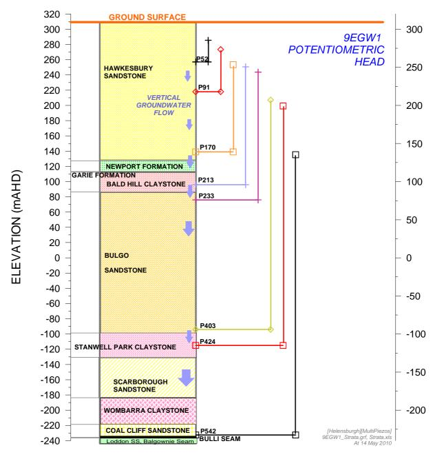
Figure 28 Vertical Groundwater Flow Directions, Relative Piezometer Elevations and Potentiometric Heads at Bore 9EGW1B [at 14 May 2010]
