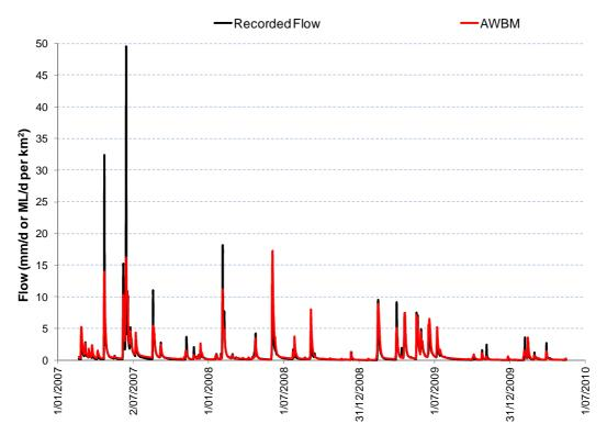
Figure 34 Recorded and Modelled Streamflow Hydrographs – GS2132102 Waratah Rivulet
