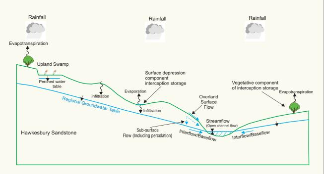
Schematic Representation of Conceptual Hydrological Model
