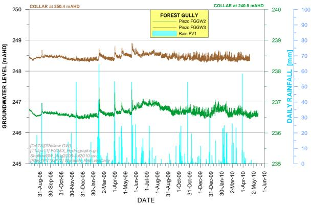
Figure 22b Shallow Groundwater Hydrographs along Forest Gully at FGGW2 and FGGW3
