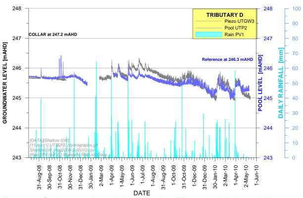
Figure 21c Shallow Groundwater Hydrographs along Tributary D at UTGW3 and UTP2
