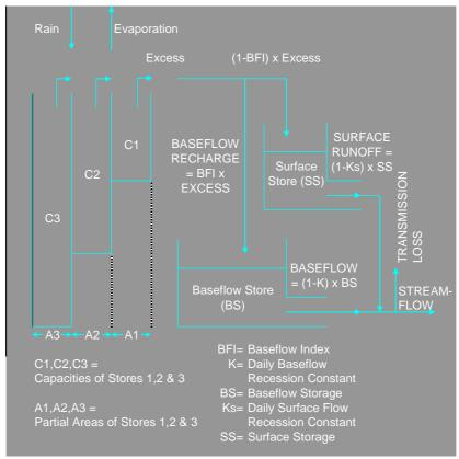
Figure 33 AWBM Model Structure and Parameter Definition
