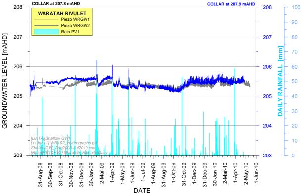
Figure 20a Shallow Groundwater Hydrographs along Waratah Rivulet at WRGW1 and WRGW2
