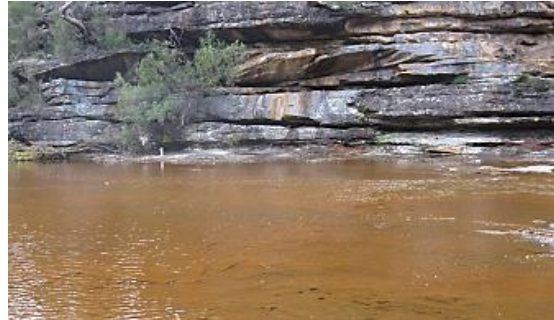
Creek Bed Iron Staining at Cliff COH1 (Downstream of Flat Rock Crossing) due to LWs 20-21
