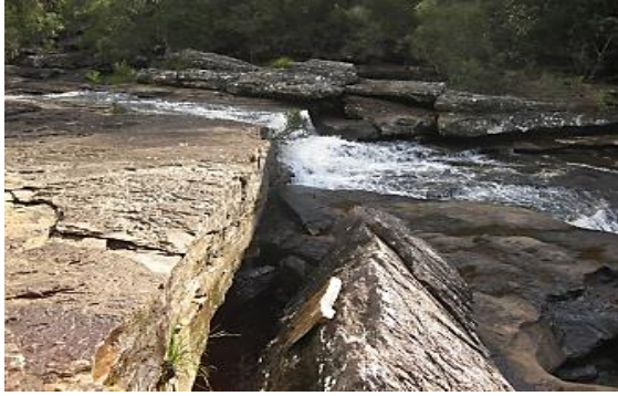
Activated Joint & Bedding Shear on Rock Bar at Pool N across Waratah Rivulet above LW 21 (downstream from Flat Rock Crossing)
