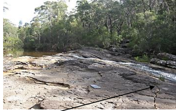
Tensile Cracking on Rock Bar at Pool N across Waratah Rivulet above LW 21 (downstream from Flat Rock Crossing)
