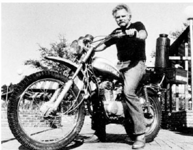
Figure 8.5.1 Old fashioned motor cycle with onboard syngas generator
