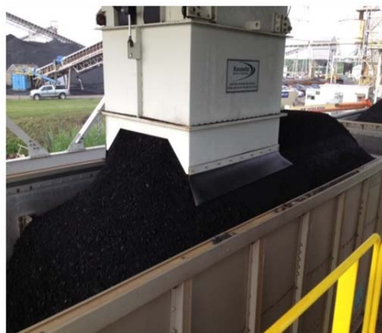
The new load out system at Gateway North reduced the time needed to load a train by as much as 67 percent.
