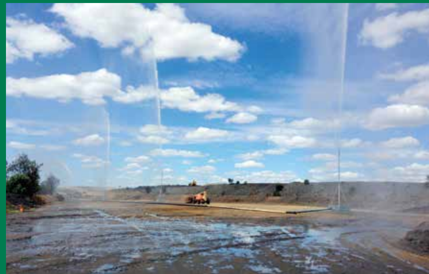
The Coppabella Mine spray misters use recycled water to reduce dust in the workshop area.
