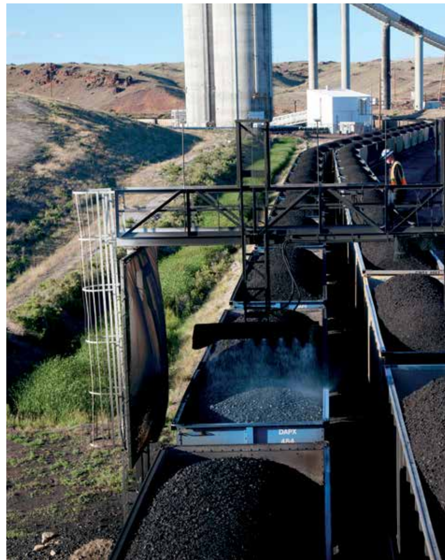
Train cars exiting the North Antelope Rochelle Mine in Wyoming are sprayed with a sealant with the same active ingredient as household glue. This dust-control measure offers added comfort to communities that host coal trains and is in use at mines from Queensland to Wyoming.
