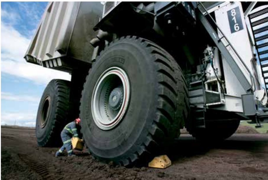
A worker at the North Antelope Rochelle Mine in Wyoming “chocks,” or backstops, the tire of a 420-ton haul truck to prevent unintended movement of the massive machine. This is one of the many rigorous practices that continue to result in improved safety at Peabody Energy.
