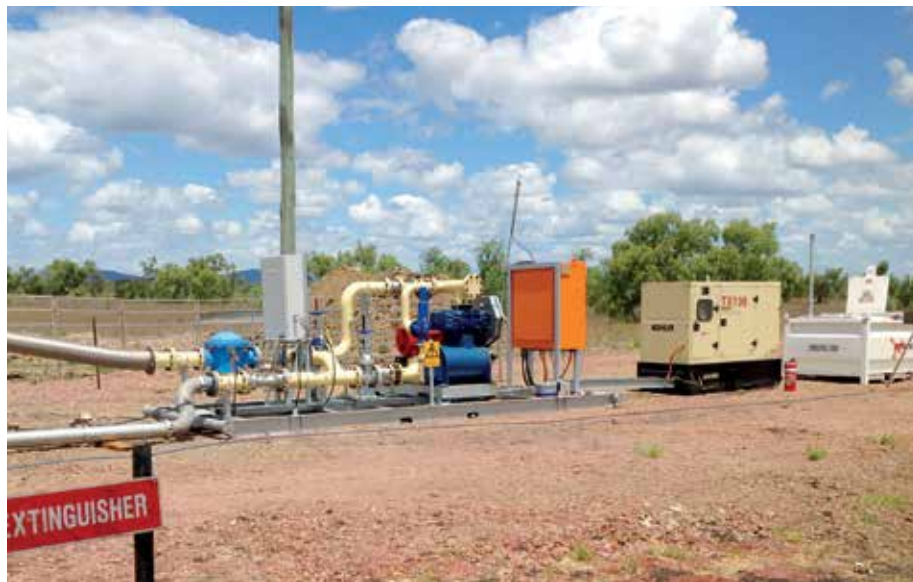
Recently installed well blowers – or Blo Skids – at the North Goonyella Mine replace less efficient methane drainage systems, saving more than 1,000,000 liters of diesel fuel per year.
