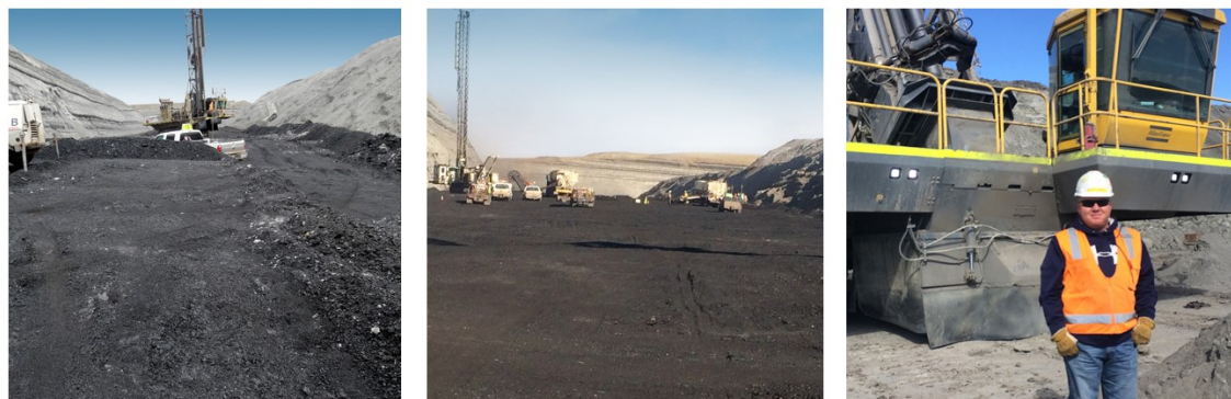
A comparison of "rough coal" (left), which contributed to coal loss and safety risks, and "smooth coal" (center) in the same pit. Top of coal is now a priority that needs to be addressed before mining operations begin at Peabody's surface mines, thanks to Jon Halverson's (right) investigation.
